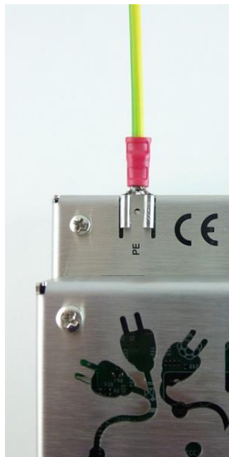
Figure 27: Grounding connection (PE) on the PiXtend V2 -L- cover
