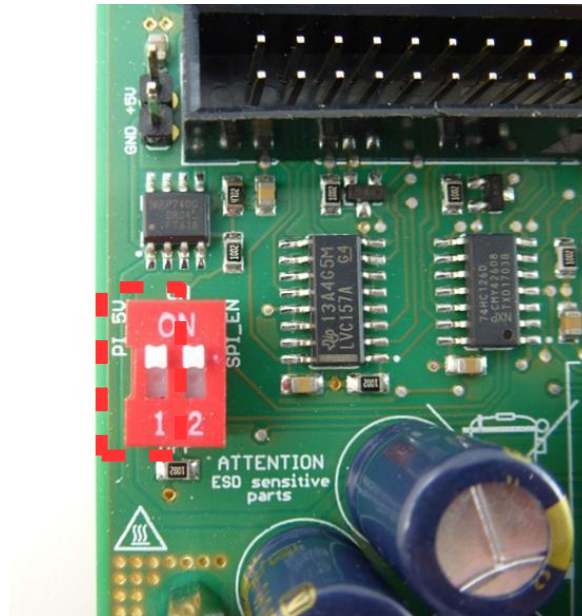
Figure 29: “PI_5V” in the “ON” position
