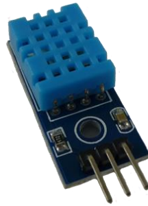
Figure 80: Temperature and humidity sensor DHT11
