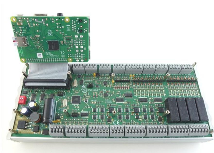
Figure 19: Raspberry Pi unscrewed from the PiXtend (ribbon cable remains connected)
