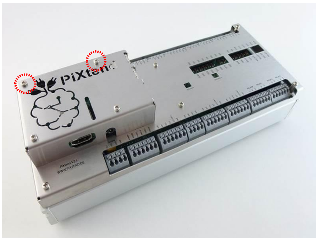
Figure 26: Completely assembled stainless-steel cover
